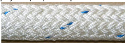
Figure 2 – Double-braided high elongation polyester (PET) 100% rope
