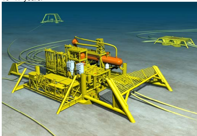
Figure 1. Illustration of the subsea separation, boosting and injection (SSBI) station. Separator and desander vessels are illustrated in orange. The
